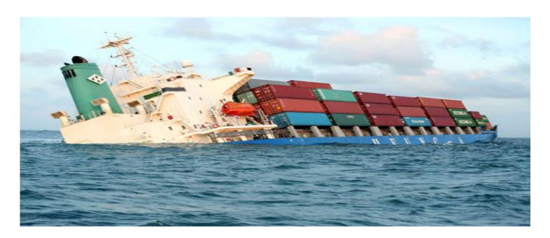
"HAD" partly sank – two holds were breached All below deck spaces flooded
